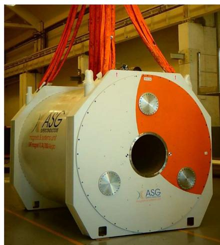
ASG Superconductors has been awarded contracts by Agilent Technologies Inc., on behalf of the USA National Institute of Health, and by the Gachon University "Gil" Medical Centre, Incheon Seoul, for the design and manufacture of two 11.74T magnet systems for applications in Magnetic Resonance Imaging (MRI) system for neuroimaging.
